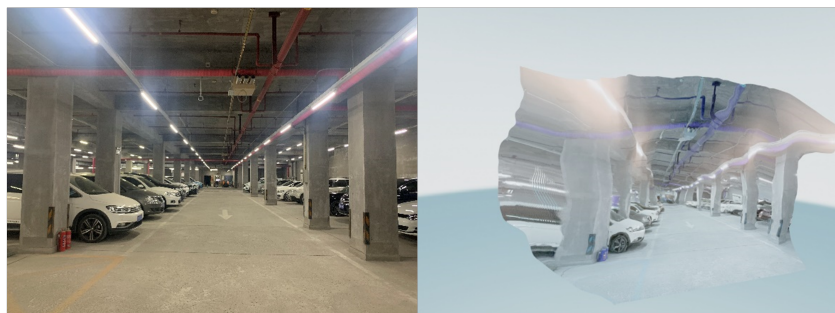
Figure 13. Modeling of point cloud arrays in corridor scenes using the Open3D tool.
