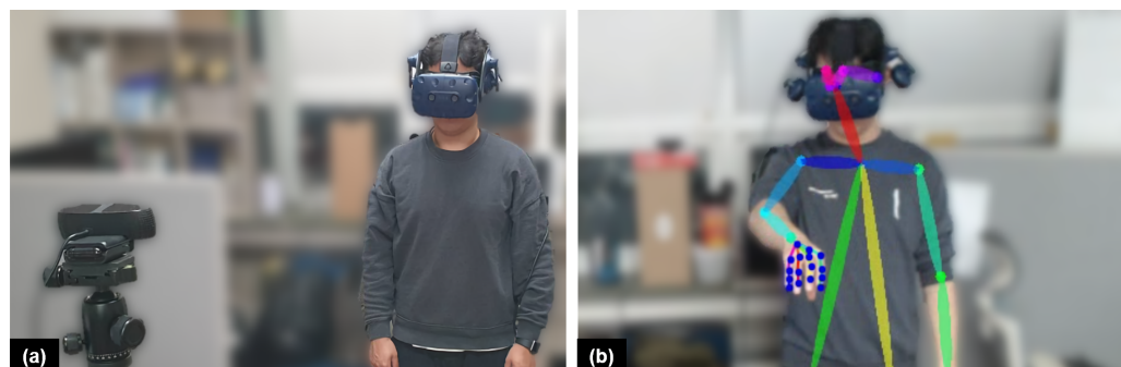
Figure 5. Setting for quantitative hand pose similarity evaluation: (a) view in third person perspective with RGB camera, and (b) estimated pose with OpenPose [43].
