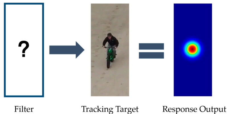
Figure 1. Correspondence between Correlation Filter Response Map and Tracking Box [7].
