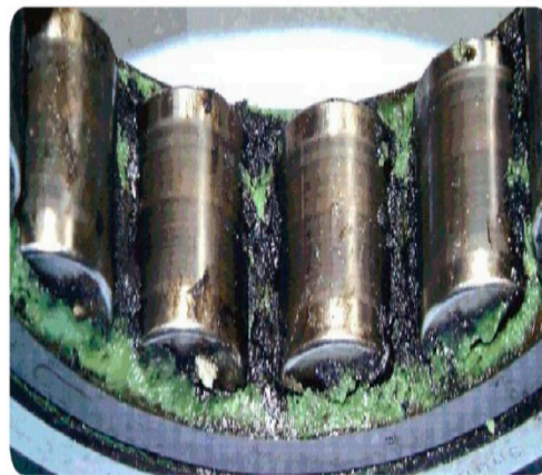
Figure 17. Bearing lubrication oil and carbonization.
