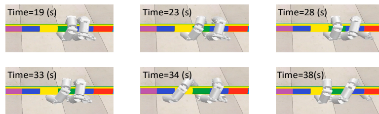
Figure 11. Snake robot change step length motion process.
