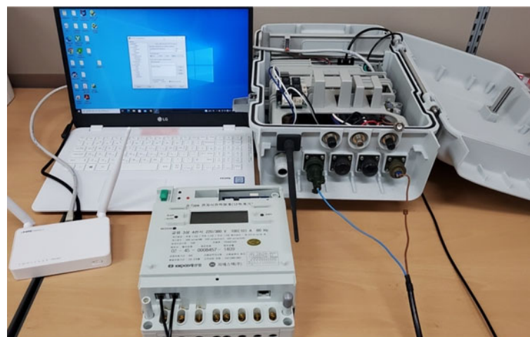
Figure 5. DCU and smart meter connected to PC based on configured test bed.
