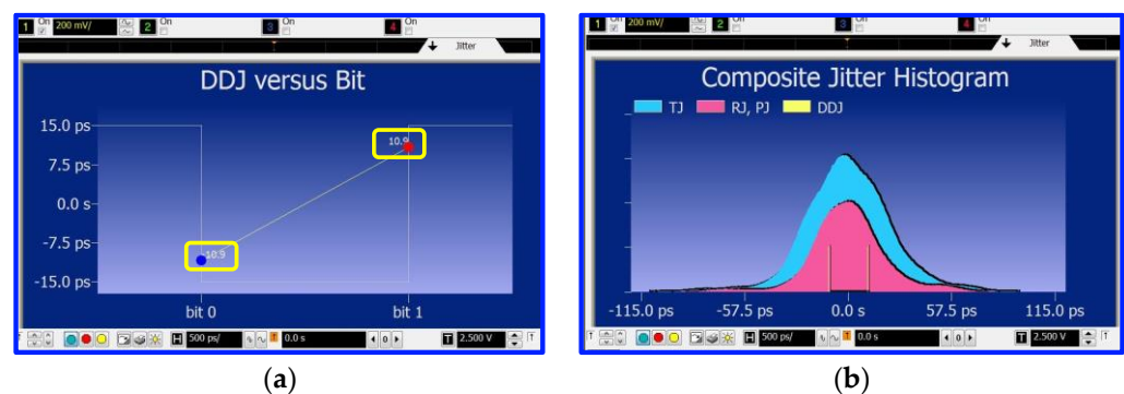
Figure 16. (a) Data-dependent jitter (DDJ) vs. bit (first 2 bits zoomed); (b) composite jitter histogram showing the distribution of jitter in the system.
