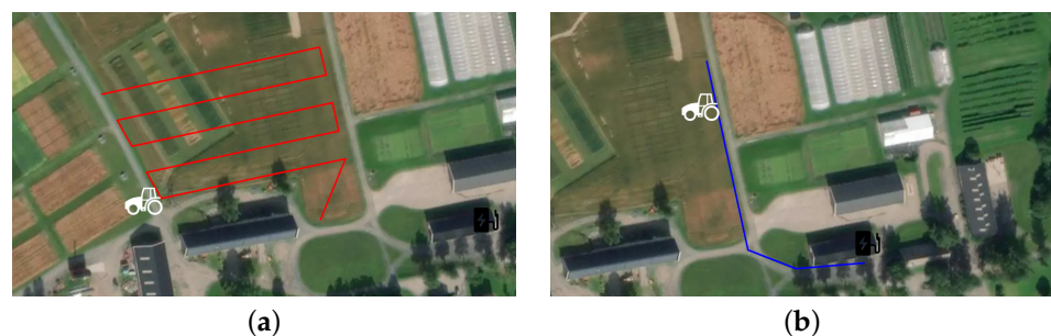
Figure 9. Two examples of the GUI control of the mobile robot. (a) Follow waypoint example. (b) Go to charging station example.
