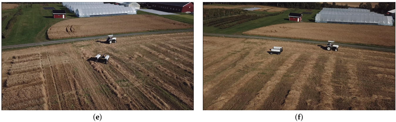
Figure 14. Experimental results of fleet navigation using a manned electric tractor and an unmanned robot tractor. (a) Field navigation sequence 1: driving in a straight line. (b) Field navigation sequence 2: approaching the headland. (c) Field navigation sequence 3: initiating a right turn. (d) Field navigation sequence 4: driving in a straight line. (e) Field navigation sequence 5: performing another right turn. (f) Field navigation sequence 6: driving in a straight line.
