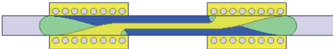
Figure 10. A back-to-back finline waveguide-to-microstrip transition structure. The grey represents the WR-10 waveguide; the yellow corresponds to the front side metal; the blue is indicative of the back side metal; the green represents the Rogers 5880 substrate.
