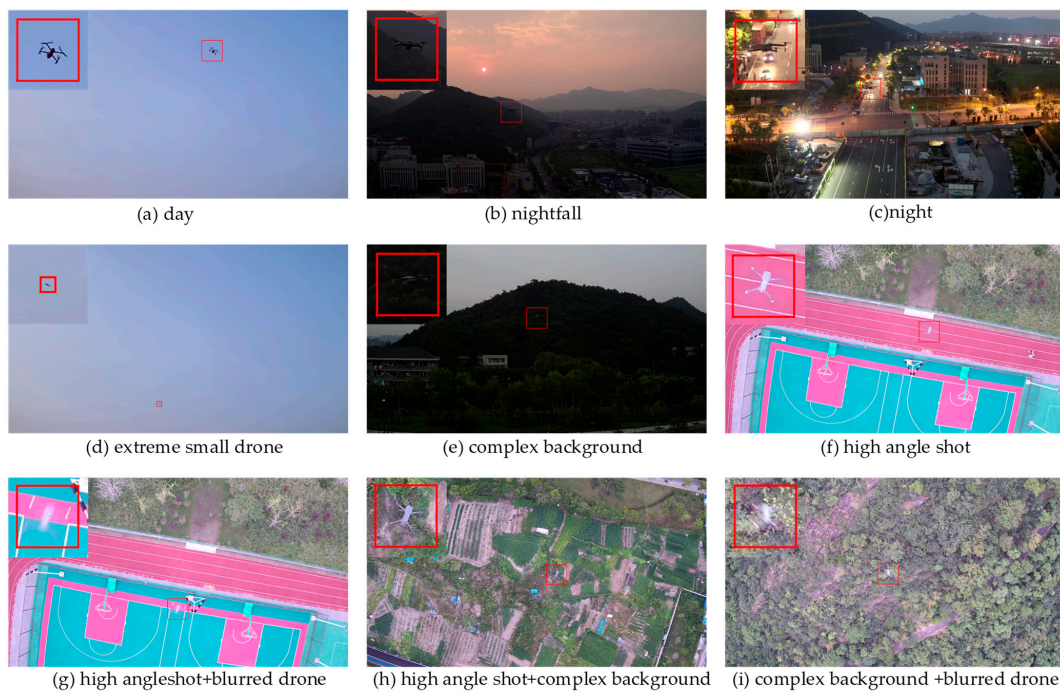
Figure 13. Selected sample plots of the self-built dataset. (a–c) show drone imagery from different time periods; (d–i) show several difficult samples, including very small drones, drones photographed from a high altitude, or complex environments.
