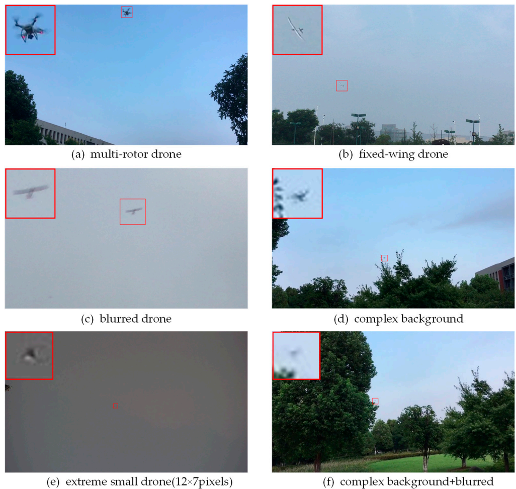
Figure 8. Display of dataset diversity. (a) multi-rotor drone; (b) fixed-wing drone; (c–f) show several difficult samples, which contain extreme small drone, blurred drone or complex environment.
