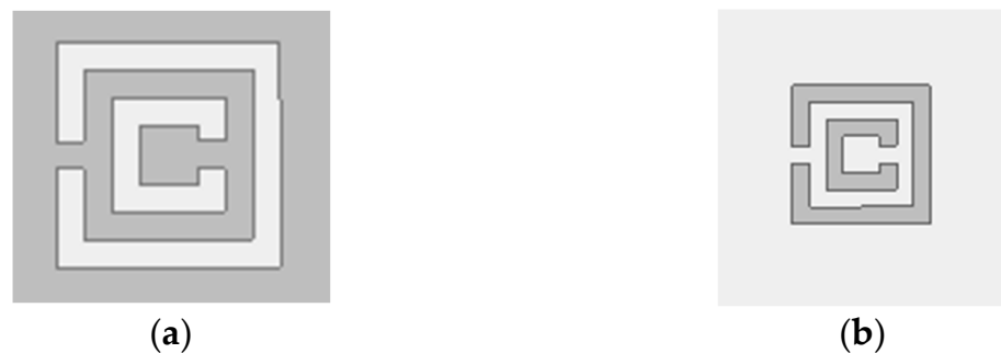
Figure 1. (a) Split-Ring Resonator (SRR); (b) Complementary Split-Ring Resonator (CSRR) (the white parts represent metal, and the gray parts represent the substrate).
