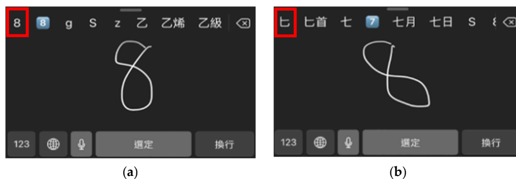
Figure 1. Handwritten digit recognition system in a mobile phone. The images in red blocks represent the recognition result of the system. (a) The system correctly recognizes the digit. (b) The system fails to recognize the digit subjected to rotations.
