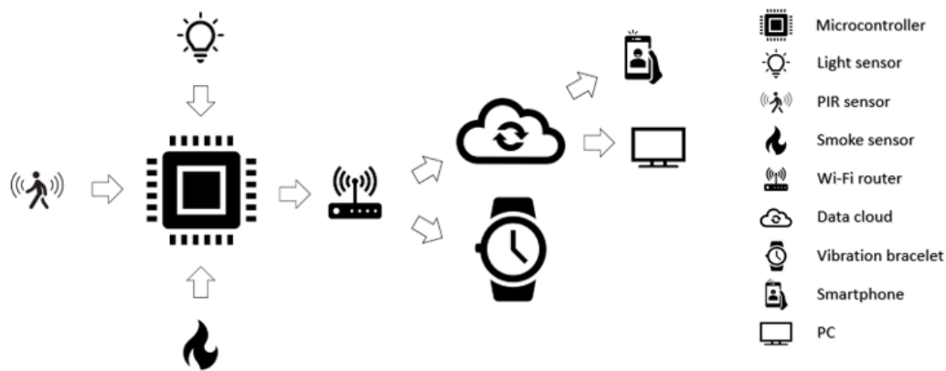
Figure 7. Block scheme of the AP-NURSE Home AP-6H version.
