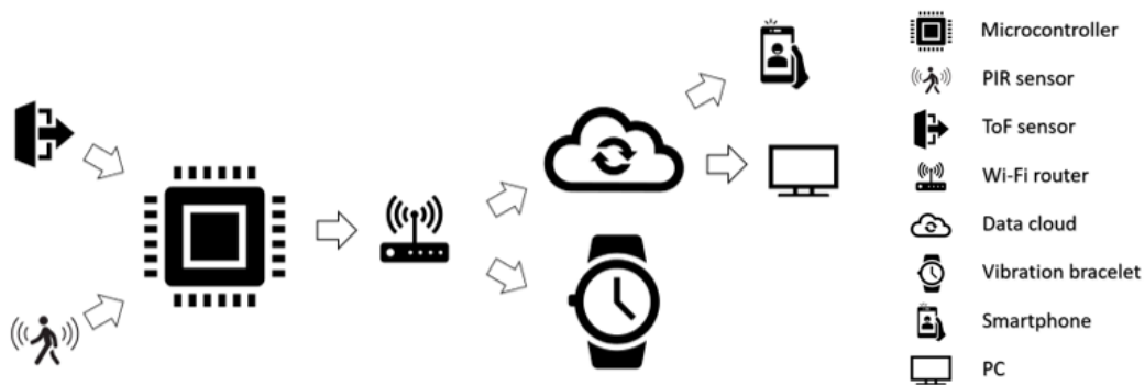
Figure 5. Block scheme of the AP-NURSE Home AP-2H version.
