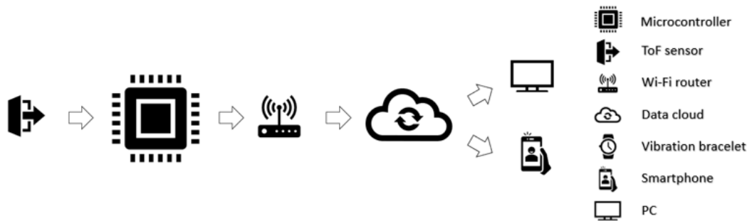
Figure 9. Block scheme of the AP-NURSE Care AP2-M version.
