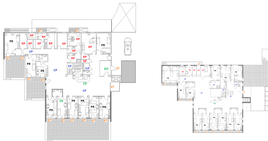
Figure 21. The building of the Social Care Centre in Bratislava. A different color means a different zone in the center and a different way of monitoring patients.
