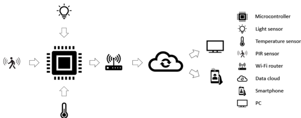
Figure 11. Block scheme of the AP-NURSE Care AP2-M version.
