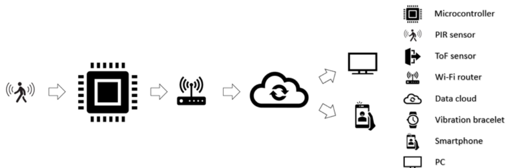
Figure 10. Block scheme of the AP-NURSE Care AP4-M and AP4-W versions.
