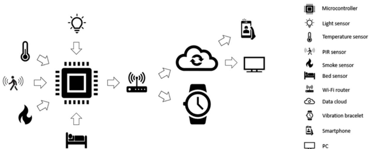
Figure 4. Block scheme of the AP-NURSE Home AP-1H version.
