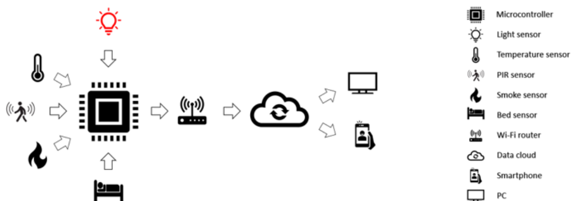
Figure 8. Block scheme of the AP-NURSE Care AP1-M and AP1-W versions.
