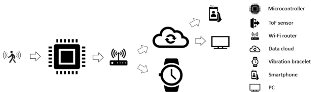
Figure 6. Block scheme of the AP-NURSE Home AP-4H version.
