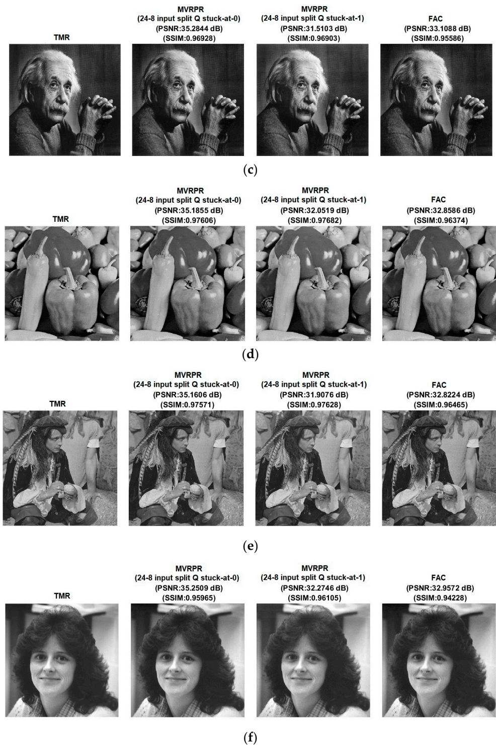
Figure 3. Results of digital image processing corresponding to TMR, MVRPR, and the proposed FAC based on experimentation with many images shown in (a–f). PSNR and SSIM values are also shown for the images. For MVRPR, a 32-bit accurate adder was optimally split into a 24-bit significant part and an 8-bit less significant part with the carry signal between these parts (Q in Figure 1b) assumed to be subject to single-bit upset as discussed in [10]. FAC is seen to consistently yield images with PSNR > 30 dB and SSIM close to unity.
