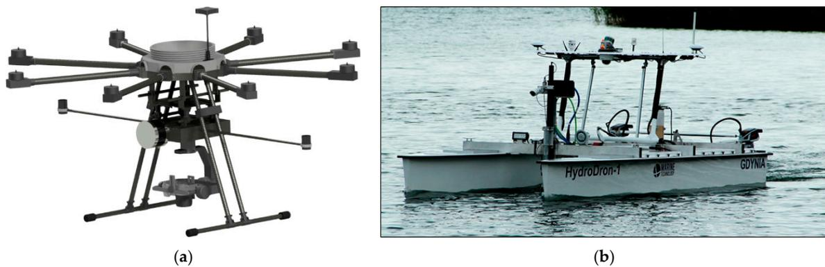
**Figure 6.** Aurelia X8 UAV with the mounted prototype optoelectronic module (a) and the “HydroDron” USV (b).
