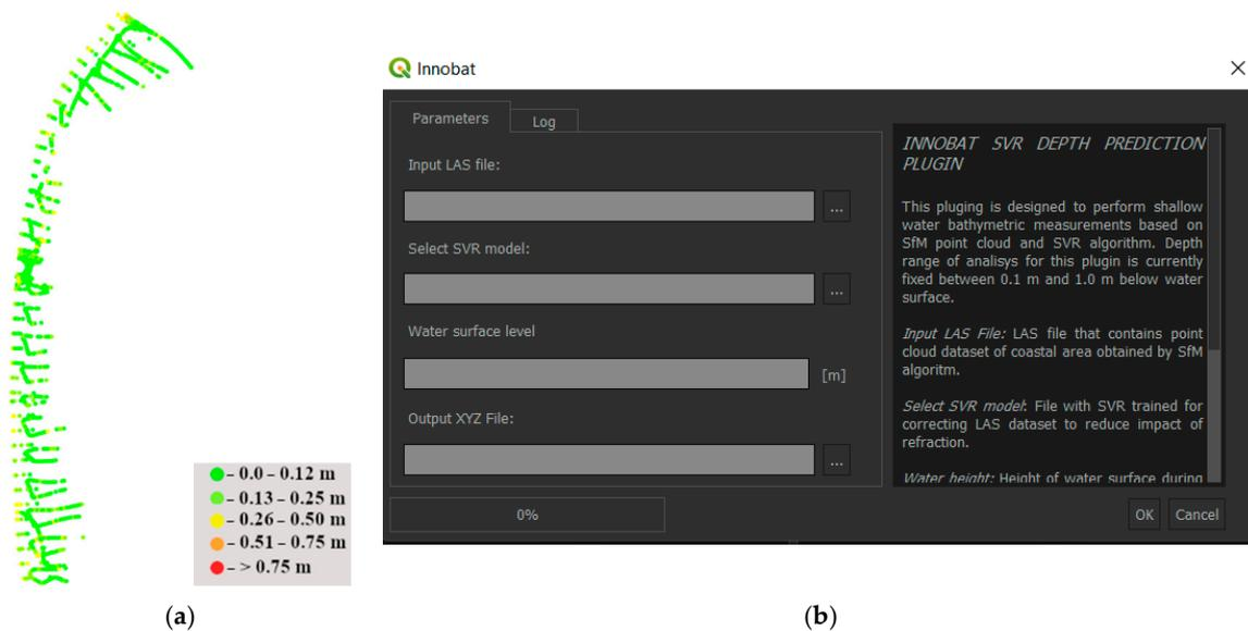
**Figure 7.** A graphic representation of the differences between the actual depths and the depths obtained by using the SVR algorithm for the depth range of 0.1 m to 1 m on the waterbody at the public beach in Gdynia (a) [52] and the user interface of the “Depth prediction” plug-in in the QGIS software (b).
