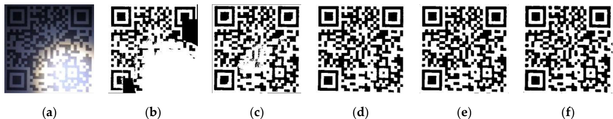
Figure 11. The QR code image with a mixture of strong local illumination and weak local illumination (Type III) and its processing by using various methods: (a) original image; (b) Yao et al. [11]; (c) Di et al. [10]; (d) Chen et al. [13]; (e) Chen et al. [14]; (f) proposed method.
