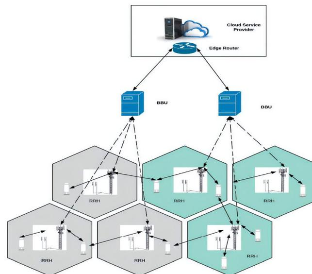
**Figure 2.** Modified C-RAN Architecture.
