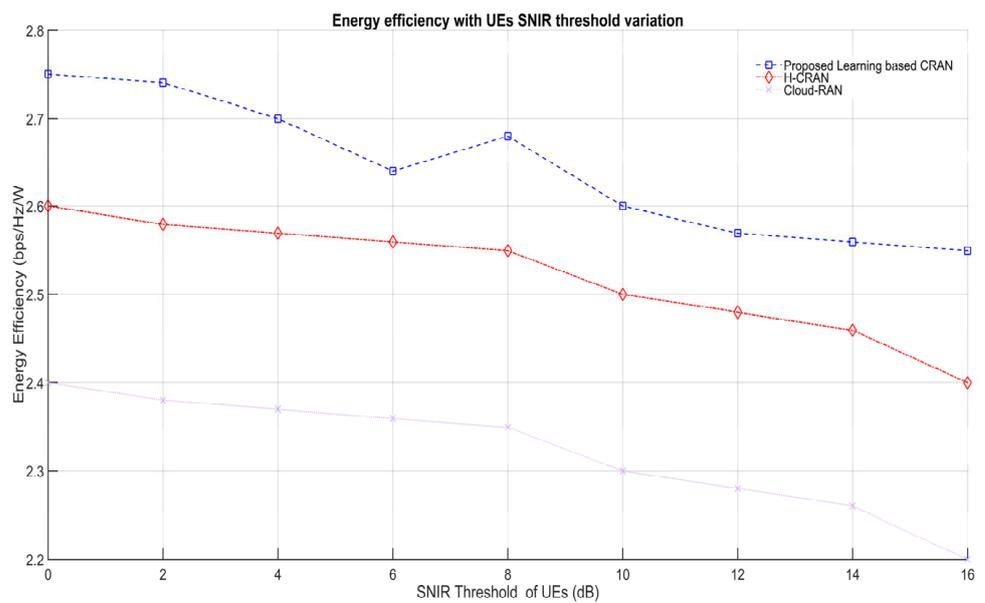
Figure 9. Energy efficiency with UE's SNIR threshold variation.
