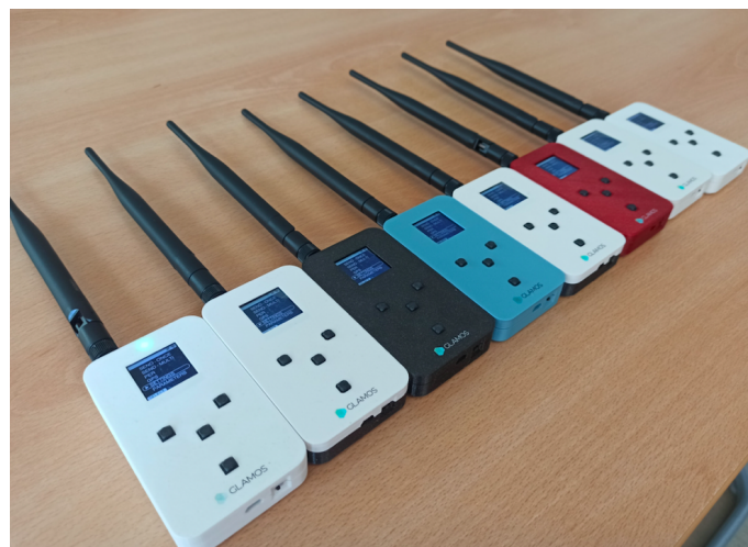
Figure 4. Glamos devices that implement ESP32 microcontroller with WiFi along with RFM95 module with for LoRa communication.
