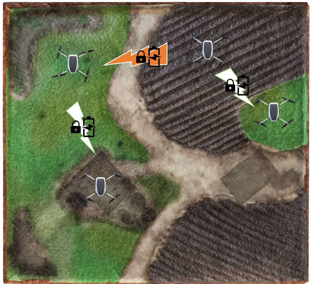
Figure 1. Illustration of a multi-robot information-gathering scenario. The links between the robots indicate the availability of communication. If all the links are present at every time, then the robots have continuous connectivity (CC). If all the links become available (or if the links create a connected network via a different topology) periodically, the robots then follow periodic connectivity (PC). On the other hand, if the white or the orange link is available, but there is no guarantee that all of them are available at any time, then we have opportunistic connectivity (OC). We want these communication protocols among the robots to be secure as well as energy-efficient.
