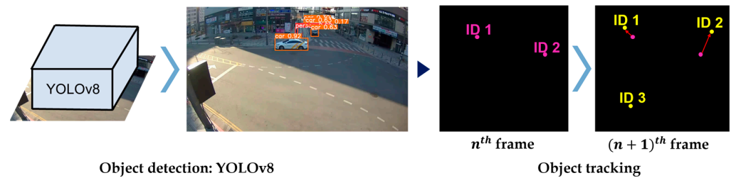
Figure 4. The procedures of object detection and tracking.
