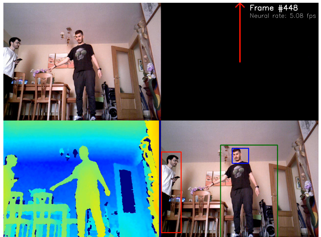
Figure 7. Output image as drawn by the program. Upper left: input RGB image. Bottom left: input depth image. Upper right: velocity commands sent to the robot and information about the neural rate and current frame number. Bottom right: tracked persons (green if it is the reference, red otherwise) and their faces (blue if it is the reference).
