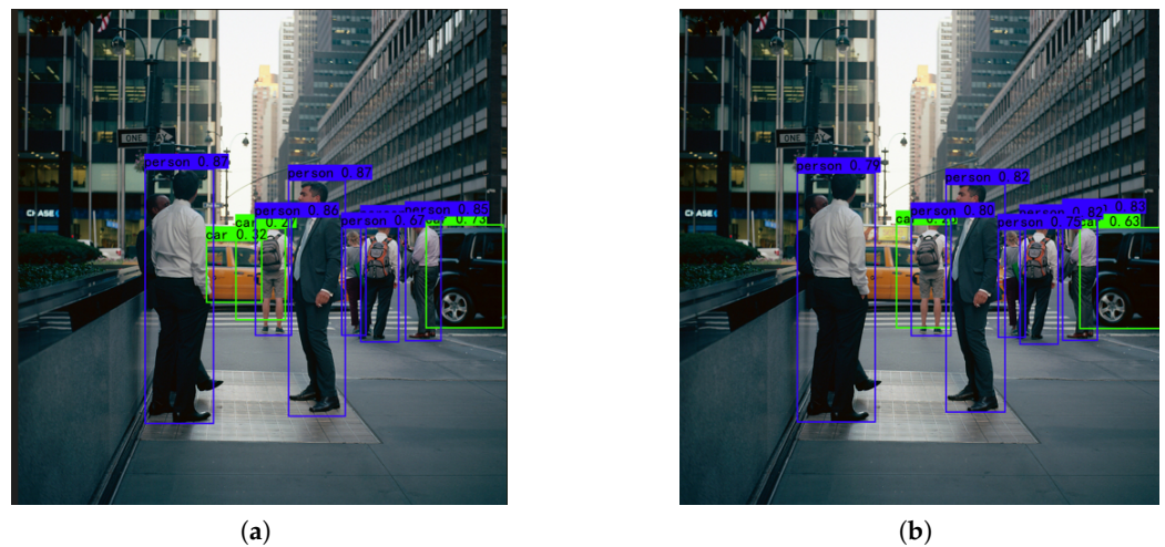
Figure 7. (a) GC-YOLO model detection results; (b) original model detection results. In this context, blue boxes indicate people, while green boxes represent cars. Compared to Figure (b), Figure (a) displays superior accuracy in identifying individuals, successfully detecting the concealed yellow car, and demonstrating an increased confidence in identifying the black car. Furthermore, there is a decreased likelihood of misidentifying a person as a vehicle.
