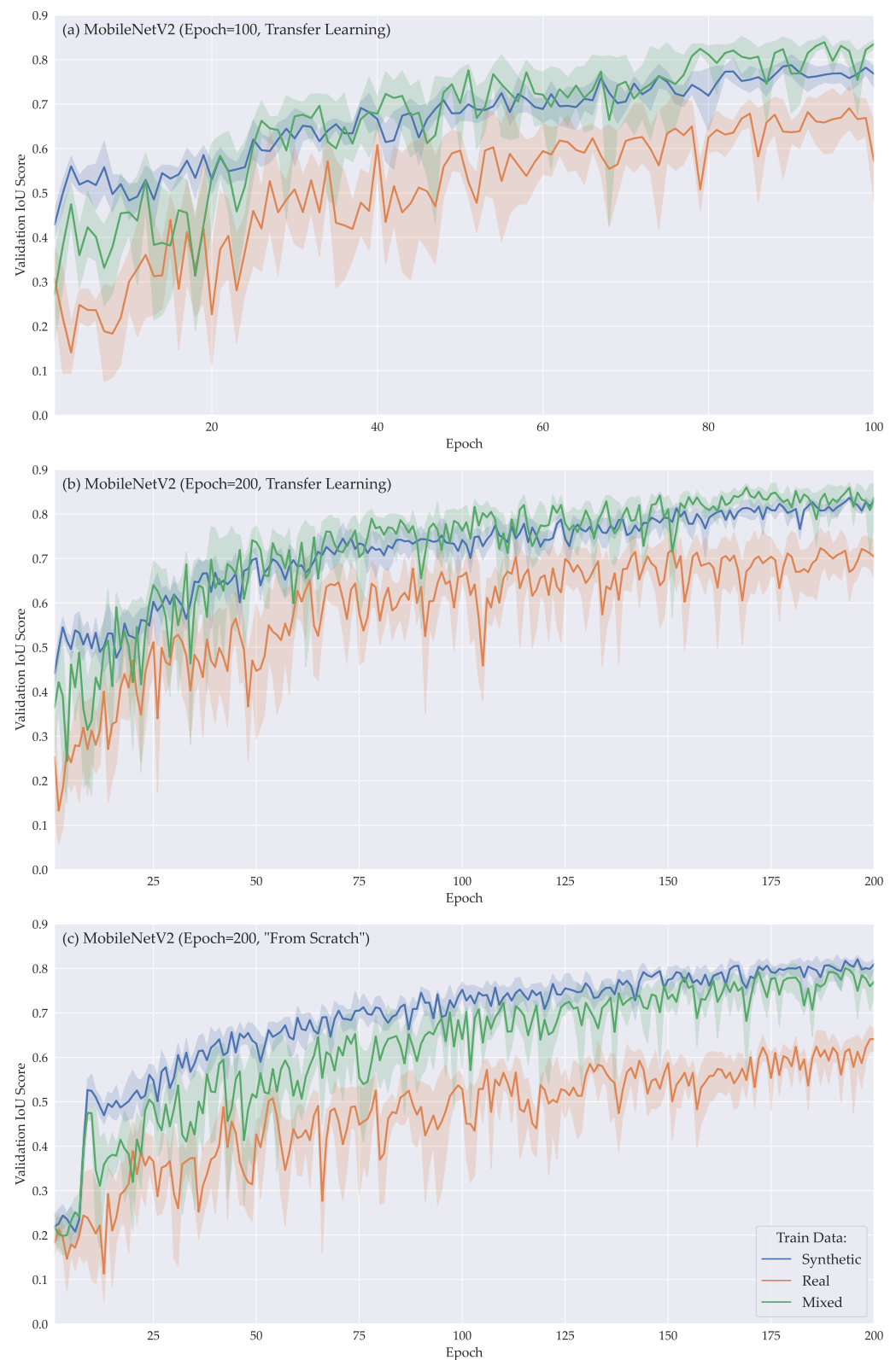
Figure 6. Results of experimental comparison of synthetic, real, and mixed datasets for the development of ruler detectors. Graphs show the dynamics of the validation IoU score during the training of the MobileNetV2 ( \alpha = 0.5 ) CNN. Training lasted for 100 epochs (a) or 200 epochs (b,c) with 500 steps per epoch; batch size: 64. Transfer learning (a) or training from scratch (b,c) was used here. Each training run was repeated five times; therefore, the graphs present the means and 95% confidence intervals depicted by translucent error bands.
