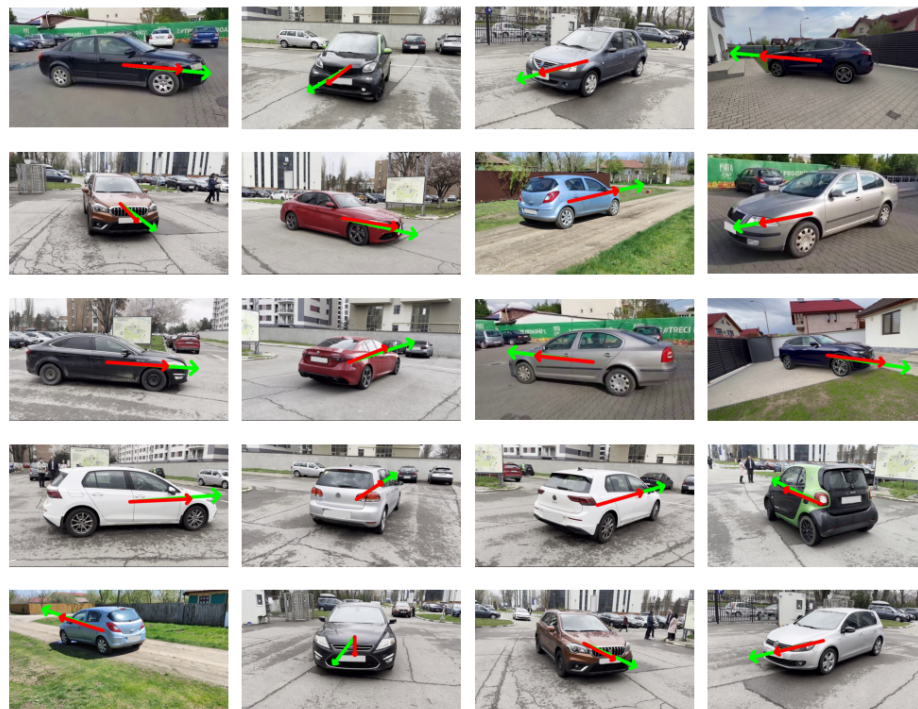
Figure 8. Predictions of the ConvNeXt model on the test set of the CFV dataset (red arrows depict the model’s predictions while green arrows show the actual labels).
