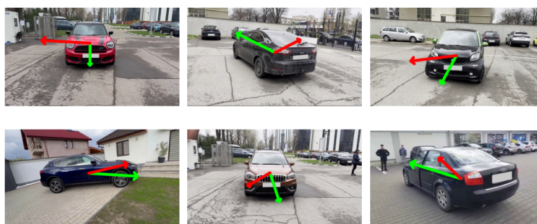
Figure 9. Samples with the highest circular absolute error (red arrows depict the model's predictions while green arrows show the actual labels).
