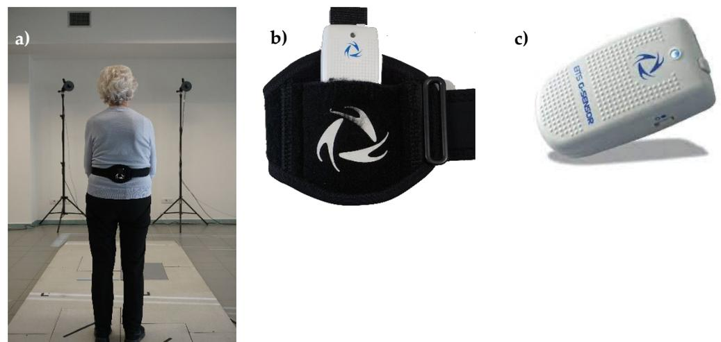
**Figure 2.** From left to right: (a) participant equipped with the IMU for the gait trials; (b) detail of the IMU positioning inside the semi-elastic belt; (c) the BTS G-Sensor IMU used for the experimental tests.
