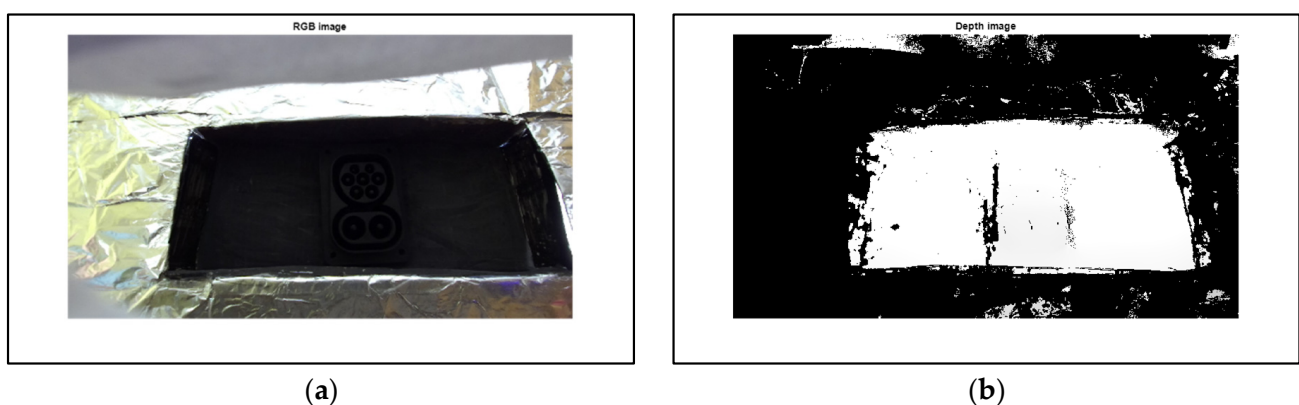
Figure 4. (a) RGB image and (b) original input depth map converted to 8-bit depth resolution.
