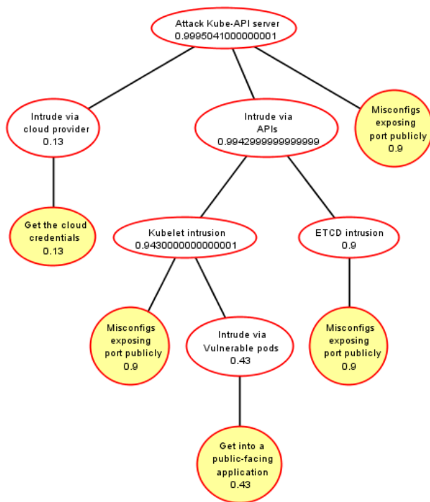
Figure 11. Probabilities in the Attack Tree for attacking the KubeAPI server.
