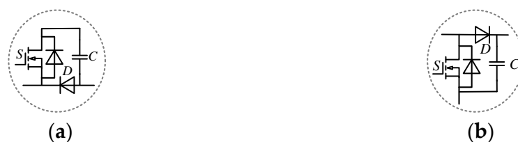
Figure 2. Two forms of the switch-capacitor cell. (a) common anode SCC. (b) common cathode SCC.
