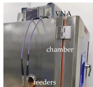
Figure 8. Photo of experiment devices used to measure thermal phase stability.
