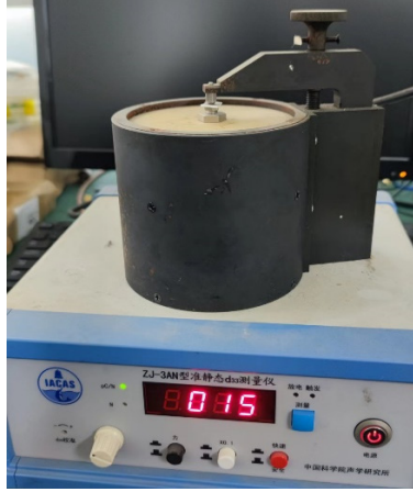
Figure S4. d_{33} test of the ZnO/PAN/Ecoflex composite membrane
