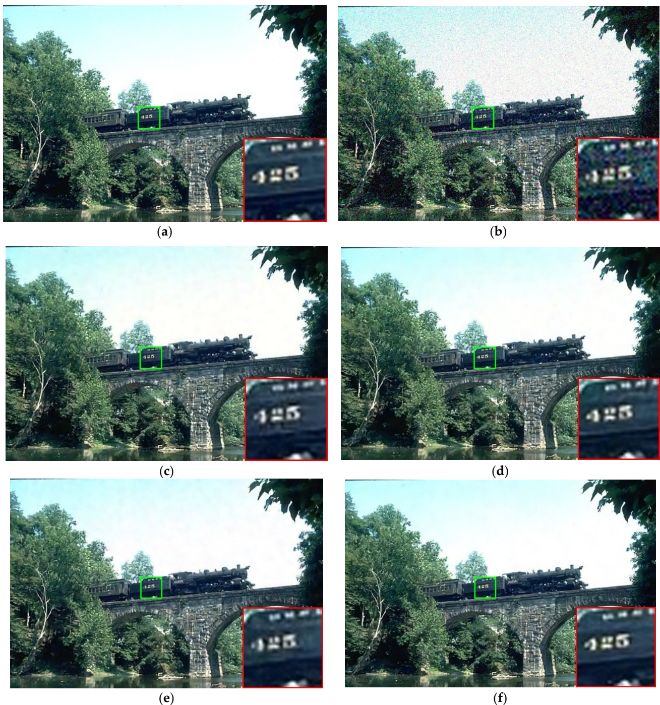
Figure 6. PSNR values of different denoising methods on one image from CBSD68 when noise level is 25. (a) Original image; (b) noisy image/16.68 dB; (c) IRCNN [12]/28.50 dB; (d) DnCNN [13]/28.81 dB; (e) ADNet [51]/28.56 dB; (f) MLIFCNN/28.86 dB.
