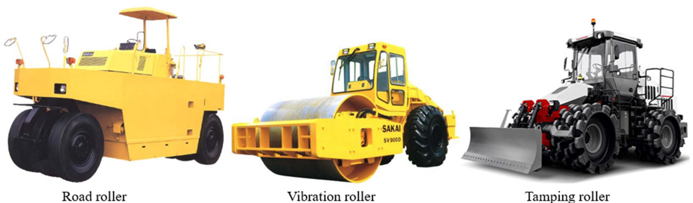
Figure 1. Three different types of rollers for construction.
