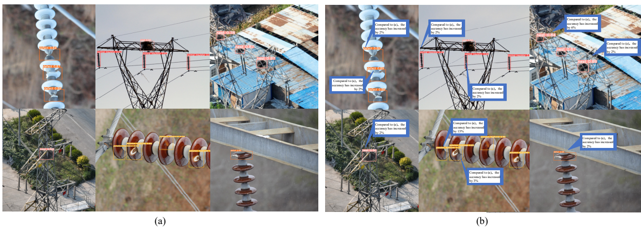
Figure 10. (a) Detection performance of YOLOv5s. (b) Detection performance of EDF-YOLOv5.
