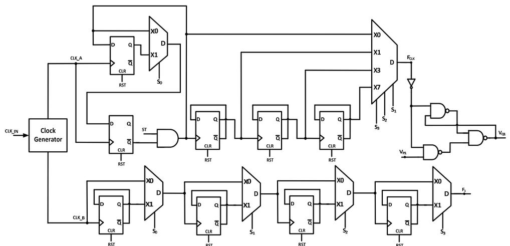
Figure 5. Proposed twin frequency control scheme (TFCS).
