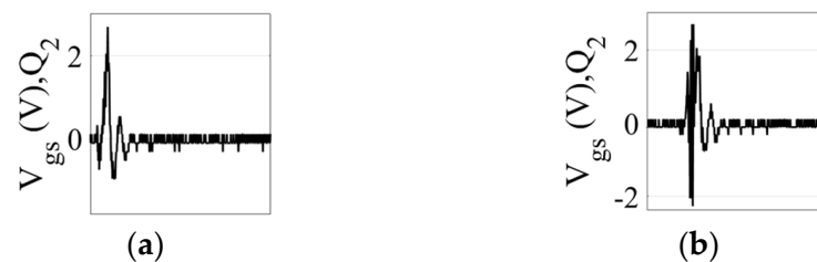
Figure 24. Enlarged view of the induced gate–source voltage of Q_2 in DPT test of case 3; (a) first turn-on of Q_1 , (b) second turn-on of Q_1 .
