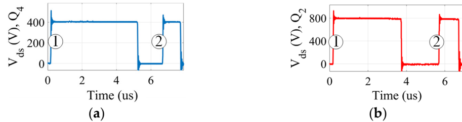
Figure 25. (a) V_{ds} and V_{gs} of the switches in case 2, and (b) V_{ds} and V_{gs} of the switches in case 3.
