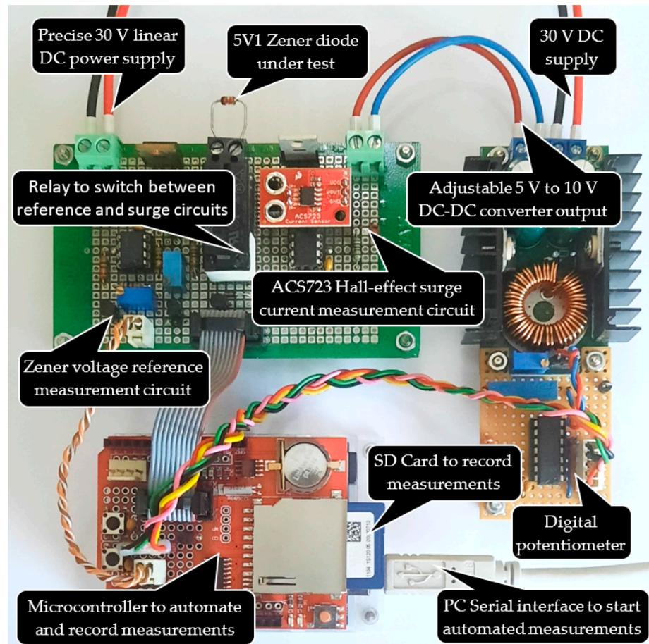
Figure 8. Actual constructed experimental test stand setup.
