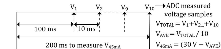
**Figure 5.** Average CCS voltage measurement and Zener reference voltage calculation.
