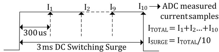
Figure 7. Average surge current level measurement and calculation.
