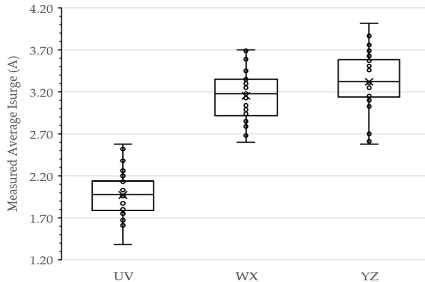
**Figure 12.** Side-by-side boxplot of the Zener diode samples: UV, WX, and YZ.
