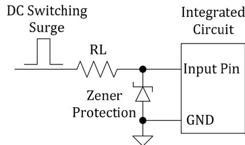
**Figure 1.** Zener diode DC switching surge protection for IC pins.
