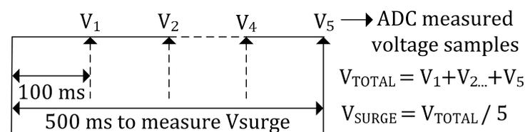
Figure 3. Average surge voltage level measurement.
