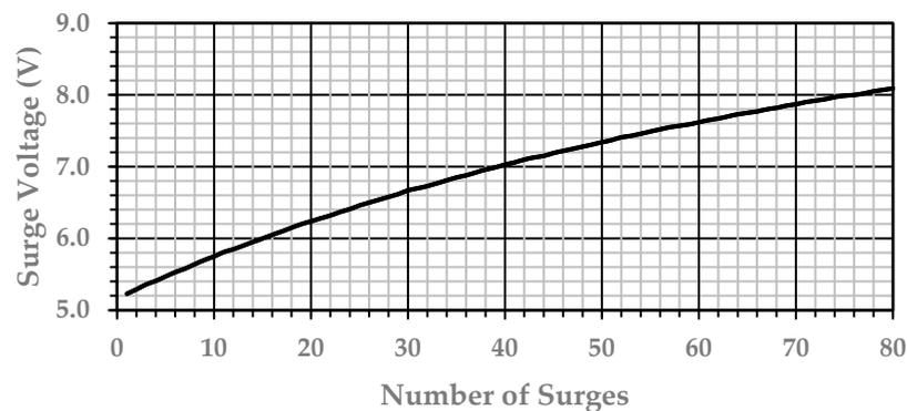
**Figure 9.** Gradual increasing surge voltage level vs. surge number.
