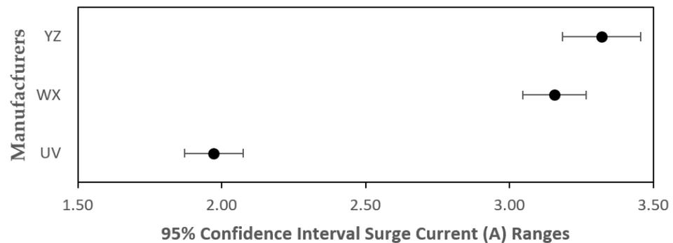
**Figure 13.** Forest plot of 95%  $C_I$  ranges of  $\overline{I_{Surge}}$  for the UV, WX, and YZ samples.
