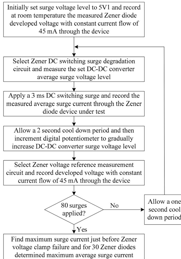
**Figure 2.** Algorithm flowchart to determine the maximum average surge current level.
