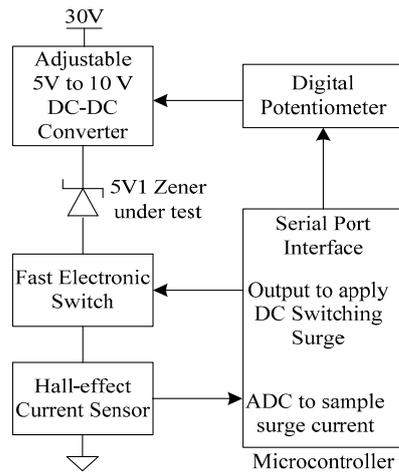
Figure 6. Zener DC switching surge current measurement circuit.
