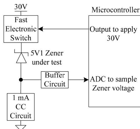
Figure 4. Zener voltage reference measurement circuit.
