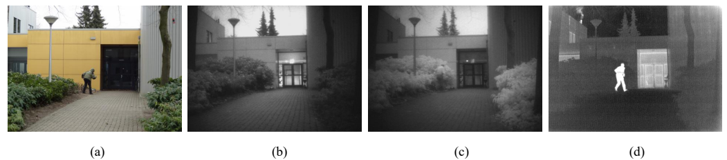
Figure 1. Multispectral images. The images are presented in the following order from left to right: (a) RGB, (b) panchromatic, (c) NIR, and (d) LWIR image. Different numbers of channels and wavelengths are the criteria for classifying these images.
