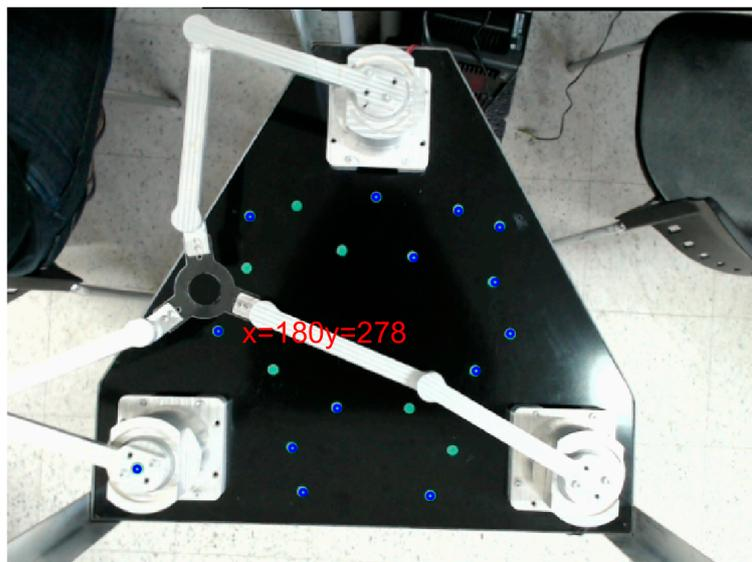
**Figure 16.** Detection of markers to determine their centroids. The blue circular sections show the centroids of each green circular element located within the manipulator’s work area, indicating the coordinates of each element.
