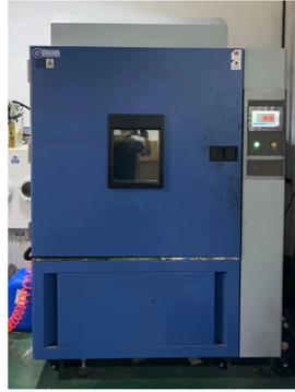
Figure 23. The high- and low-temperature test chamber.
