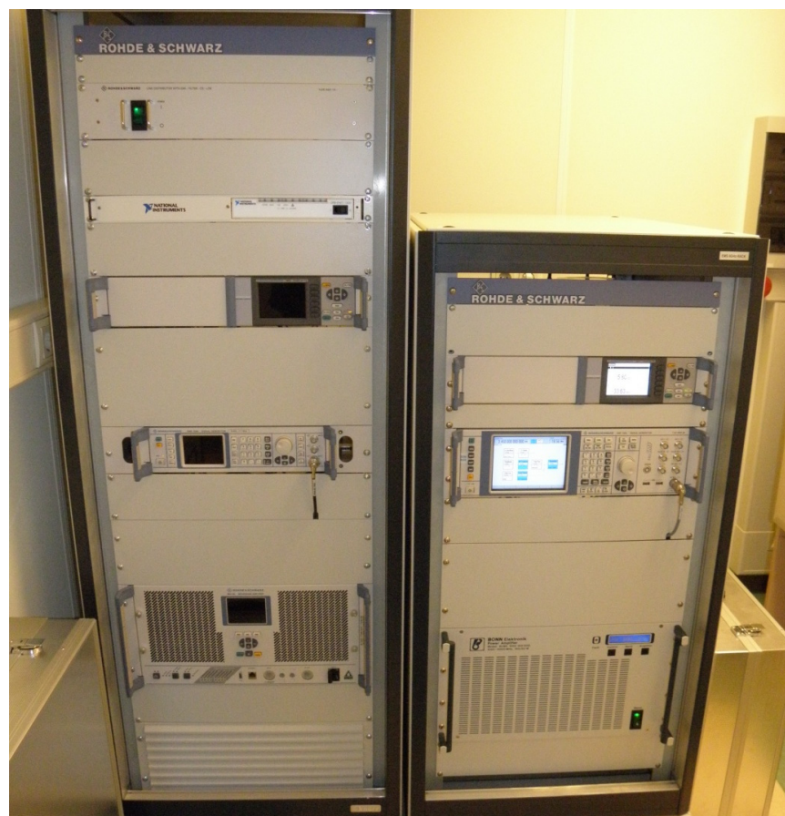
Figure 5. View of the systems (EMS_1GHz and EMS_6GHz) by Rohde & Schwarz for the generation of electromagnetic fields at the required intensities and frequencies during operation.
