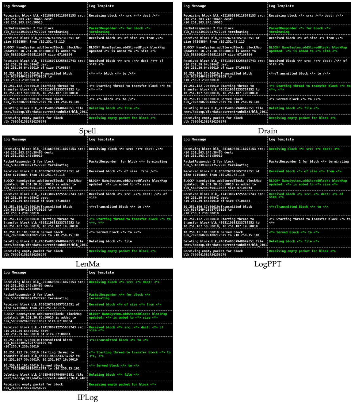
Figure 5. Comparison of parsing results of different parsing methods for ten randomly selected log messages in HDFS (green log templates represent correct parsing).
