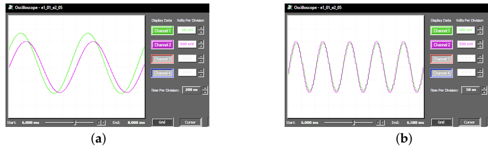
Figure 10. Input and output waveforms of the filter described by (15) for \epsilon_1 = 0.1 and \epsilon_2 = 0.5 , stimulated by (a) 1 V, 1 kHz and (b) 1 V, 10 kHz sinusoidal signal.
