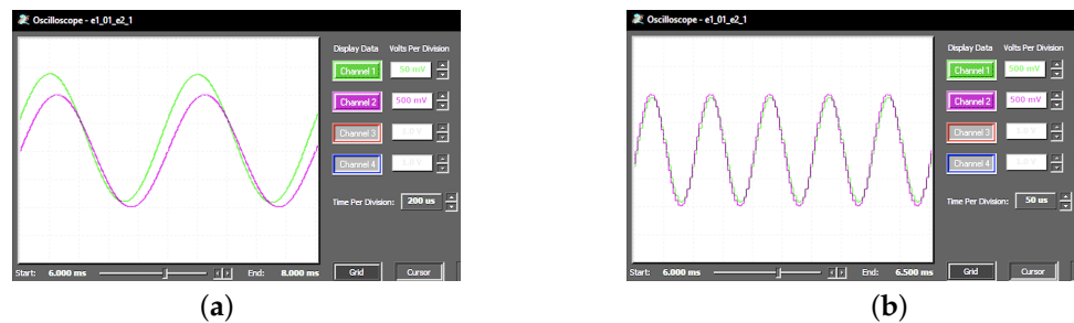
Figure 11. Input and output waveforms of the filter described by (15) for \epsilon_1 = 0.1 and \epsilon_2 = 1 , stimulated by (a) 1 V, 1 kHz and (b) 1 V, 10 kHz sinusoidal signal.
