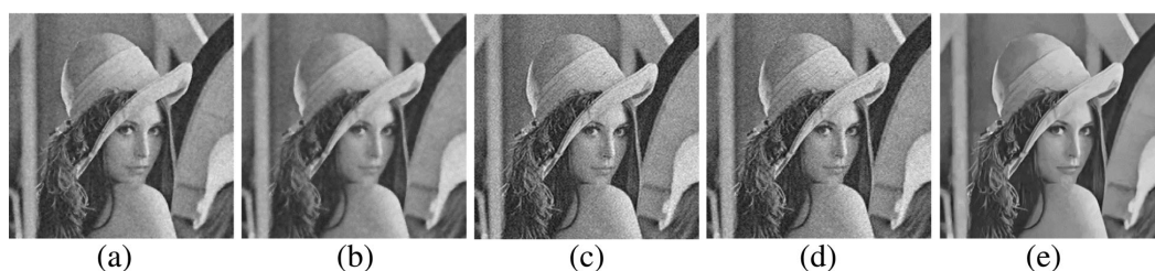
Figure 1. Visual comparison of denoising methods using the Lena image with Gaussian noise ( \sigma = 30 ): (a) Wiener filter (PSNR: 27.81; SSIM: 0.707); (b) bilateral filter (PSNR: 27.88; SSIM: 0.712); (c) PCA (PSNR: 26.68; SSIM: 0.596); (d) wavelet transform (PSNR: 21.74; SSIM: 0.316); (e) BM3D (PSNR: 31.26; SSIM: 0.845) [8].
