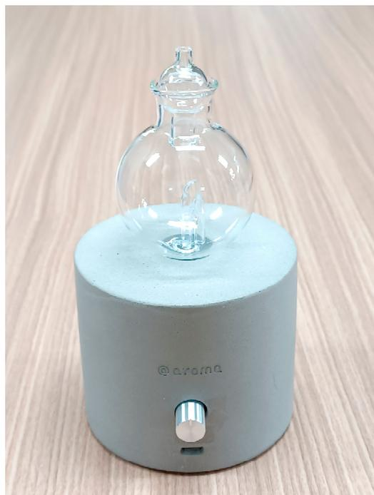
**Figure 2.** Diffuser used in the experiment. Body dimensions: 80 mm (diameter)  $\times$  152 mm (H); weight: 376 g; spray method: nebulizer; maximum diffusion capacity: 70 m<sup>2</sup>.
