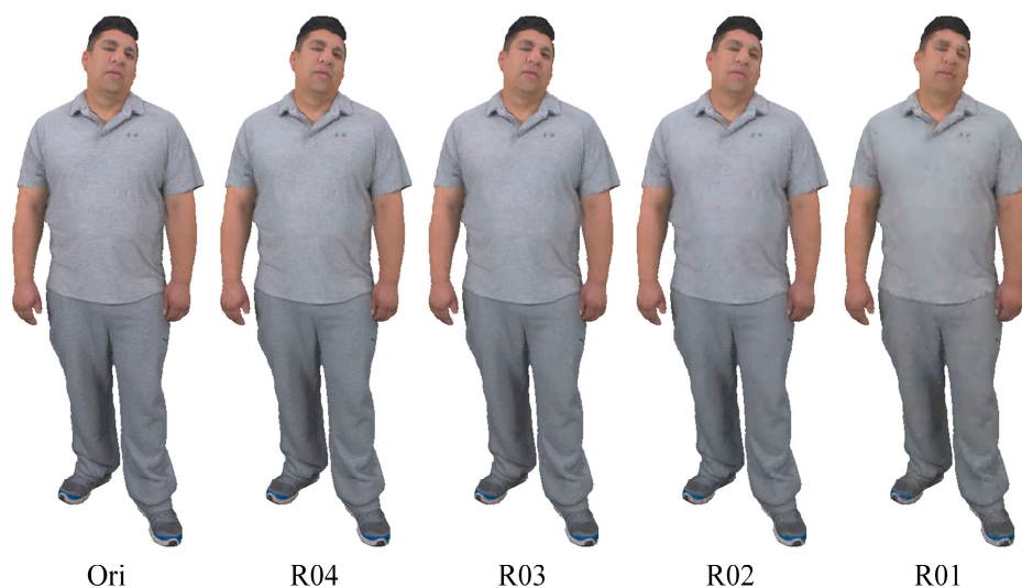
Figure 1. The “boxer_viewdep_vox12.ply” image [20] under different G-PCC attribute compression levels. First on the left: the original PC, followed by PCs compressed using G-PCC with different attribute compression levels R04, R03, R02, and R01.
