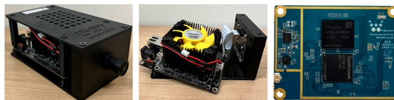
Figure 7. AI camera that includes an embedded board with Qualcomm QCS610 SoC; (left) exterior, (middle) interior, (right) embedded board inside the camera.
