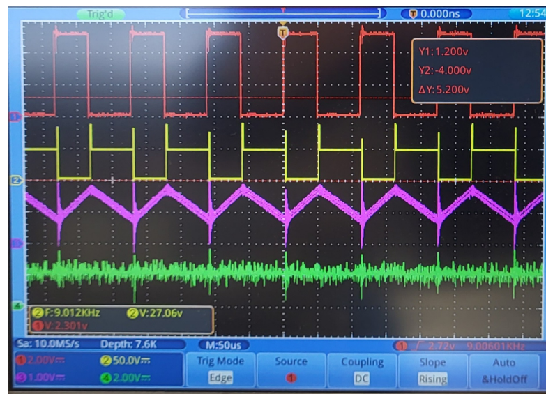
Figure 10. Signals representing the control signal applied to transistor T2 (red trace), the voltage across transistor T2 (yellow trace), the current sensor voltage from the PV array emulator (purple trace), and the voltage sensor output from the PV array emulator (green trace). All signals are measured in V.
