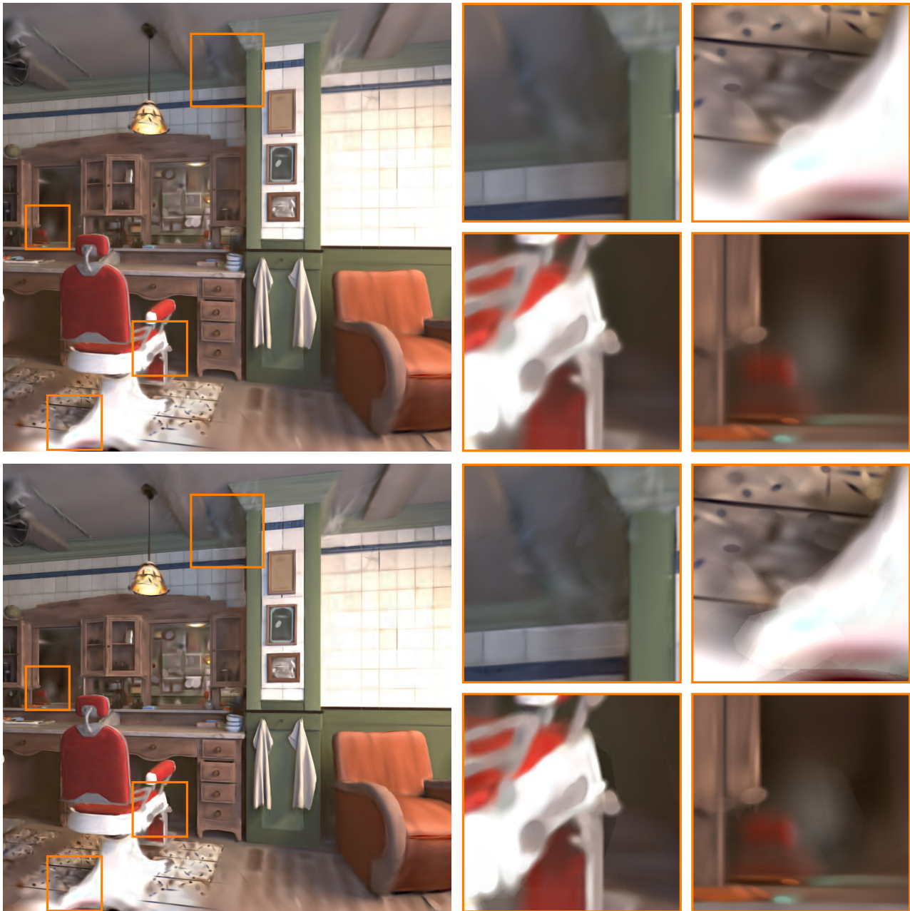
Figure 3. The highest-quality render with \bar{\alpha} = 0.125/256 ( top ), compared to the lowest-quality render with \bar{\alpha} = 15/256 ( bottom ), of the tilted view in the test of Figure 2. These results were produced in 4.1 ms and 2.2 ms, respectively. The quality of the fastest render (i.e., highest \bar{\alpha} , bottom ) is still relatively high (i.e., 39 dB instead of 59 dB). The most noticeable artifacts have been highlighted. Notice how the regions of influence of components being cut off too early cause sharp edges for smooth components (i.e., low s_i ). This effect is less noticeable for components that already have a sharp edge.
