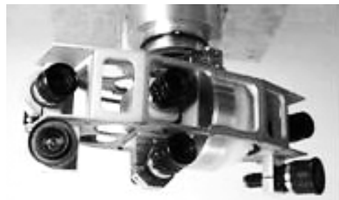
Figure 6. Camera set used in VaMoRs in the AutoNav-project 1997–2003 with two pairs of stereo-cameras (parallel, outside top and divergent looking, bottom).
