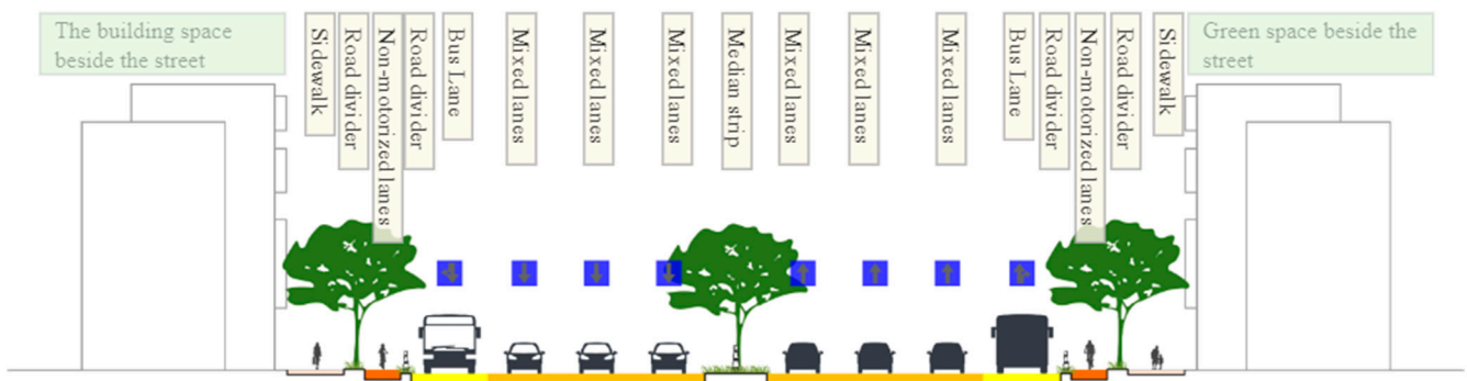
Figure 12. Typical street section mode of Beijing Road.
